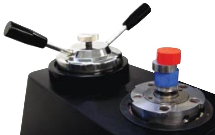
*Duplexing spacer provided with each mold assembly allows 2 mounts to be produced per cycle. Bayonet cap rests on a convenient heat-sink/holding tray between cycles.*
