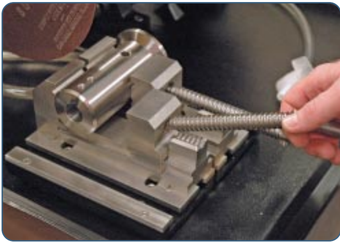
Dual vises allow burr-free cutting
